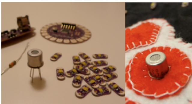
Figure 2. Parts used for the prototype: battery holder, Lilypad Arduino, LEDs, VOC sensor, resistor (from top left, clockwise, left) and the VOC sensor attached on a T-shirt (right)
