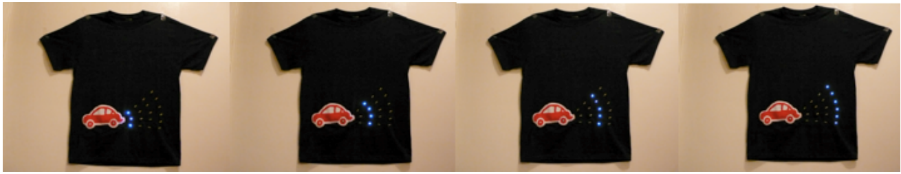
Figure 1. WearAir, a lightening T-shirt. Four arrays of LEDs lighten in a sequence from left to right.
